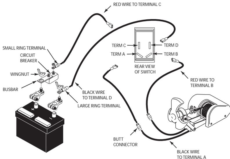
Figure 2. Deckmate 19 Wiring
